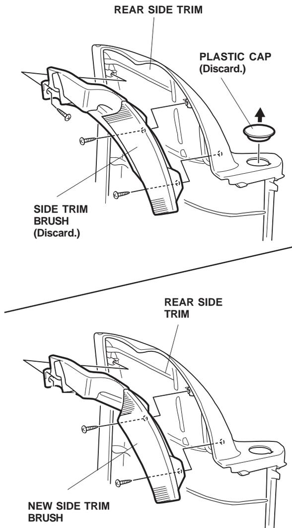
12. Get the right rear side trim, removed in step 5. Repeat step 11 to install the new right side trim brush to the right rear side trim.
